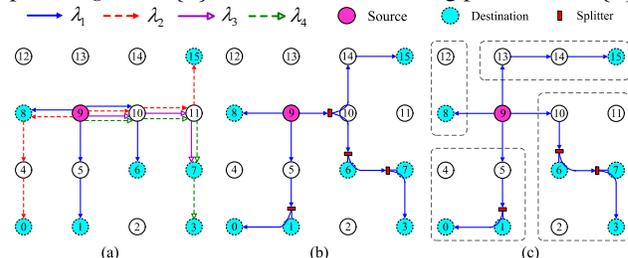
Fig. 2. Replication-based multicast routing schemes for a  $4 \times 4$  ONoC, (a) unicast-based scheme with exclusive wavelengths assignment; (b) tree-based and (c) path-based schemes with optical splitters.
