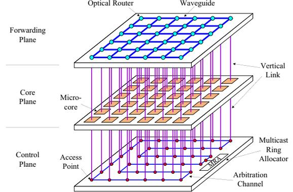
Fig. 4. Network architecture with three logical planes: core plane (micro-cores), control plane (centralized multicast ring/wavelength allocation), and forwarding plane (multicast packet delivery).
