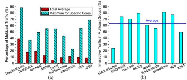
Fig. 1. Analysis of multicast traffic in a 64-core system running PARSEC benchmarks, (a) the percentage of multicast packets for each core; (b) the average percentage of interactive multicast packets in same multicast group.
