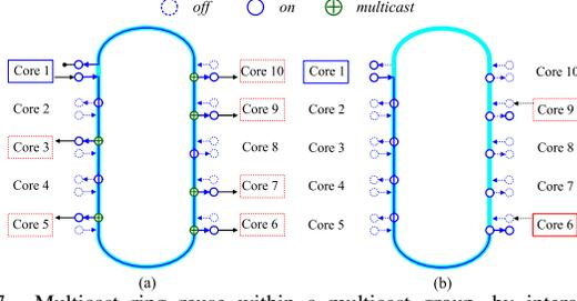
Fig. 7. Multicast ring reuse within a multicast group, by interchanging between two states: (a) multicast routing, and (b) optical token arbitration.
