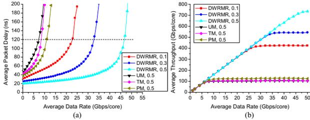
Fig. 11. Performance evaluation of multicast ring reuse for interactive multicast traffic,  $\tau = 0.1, 0.3, 0.5$ , in average (a) packet delay and (b) throughput. half number of wavelengths than other schemes. It can greatly reduce the demand of on-chip lasers, E/O&O/E converters, and microring resonators. Due to the complexity of optical devices, this reduction is more considerable compared to the hardware cost on recording multicast rings and wavelengths.
