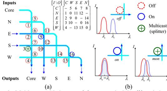
Fig. 6. Multicast-enabled router, (a) router principle; (b) switch status. multicast ring both considering the minimization of peak wavelength utilization and the length of multicast ring, to accommodate as many multicast rings as possible with limited wavelengths. When a multicast ring is allocated, MRA updates the global wavelength table and sends out configuration packets.
