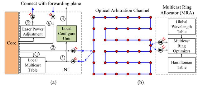
Fig. 5. Main components and communication process in (a) core plane (local configuration), and (b) control plane (centralized allocation).
