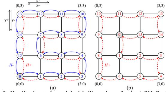
Fig. 8. Hamiltonian cycles and the labelling scheme for  $4 \times 4$  ONoC, starting from the source core of (a)  $(x_s, y_s) = (0, 0)$  in  $H^-$ , and (b)  $(x_s, y_s) = (1, 2)$  in  $H^+$ , respectively.
