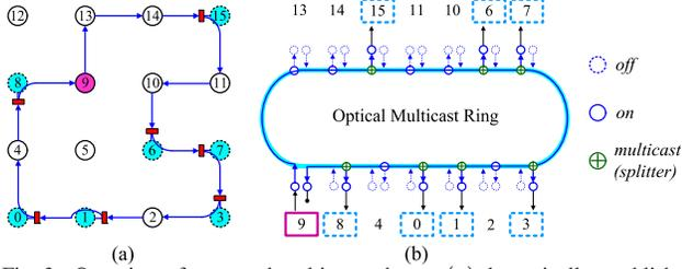
Fig. 3. Overview of proposed multicast scheme, (a) dynamically established multicast ring for routing; (b) single-send-multi-receive transmission.
