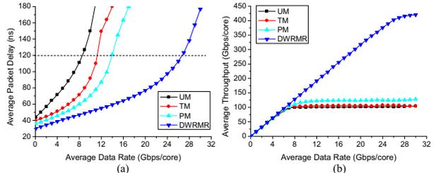
Fig. 9. Comparison with different schemes, unicast-bast (UM), tree-based (TM), and path-based (PM), in average (a) packet delay and (b) throughput.
