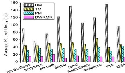
Fig. 12. Average multicast packet delay in trace-based simulations.
