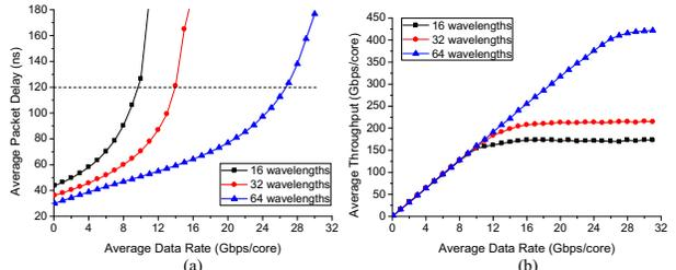
Fig. 10. Performance evaluation with different number of wavelength channels for DWRMR, in average (a) packet delay and (b) throughput.
